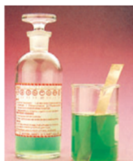
Figure 2 When a strip of copper is placed in a solution of nickel(II) ions, the green nickel(II) ion colour remains and the copper metal does not react. Collisions between copper atoms and nickel(II) ions apparently do not result in the transfer of electrons.
