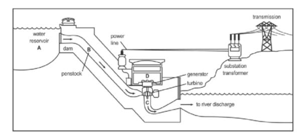
34. The efficiency of a hydroelectric dam is calculated by the ratio of the output energy divided by the input energy of the water in the reservoir. Identify the output and the input forms of energy as shown in the diagram above.
